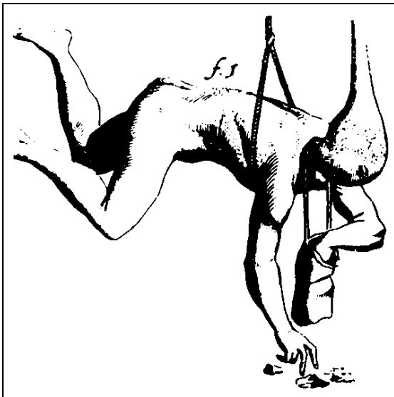
Figure 1-1. Early Impractical Breathing Device. This 1511 design shows the diver's head encased in a leather bag with a breathing tube extending to the surface.
